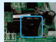
Compressor current protection
